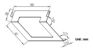
Assemble the hooks on two sides of the bracket into the groove on the rear cover of the monitor.
