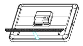
Align the edge of the silicone non-slip mat to the back of Indoor Monitor.
